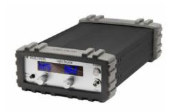
The SSFL 785 nm Spectrum Stabilized Fiber Coupled Laser Source provides a powerful and extremely stable laser source that is ideal for scientific applications including Raman Spectroscopy. The unit contains a fiber-coupled high-power diode that is spectrally narrowed and wavelength-stabilized by incorporating a Volume Bragg Grating (VGB). It outputs over 300 mW and 500mW at 785 nm laser having wavelength stabilized within 0.5 nm.
